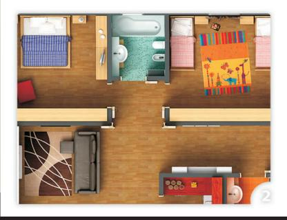
Layout 1 a floor plan using normal swinging door. Layout 2 COMPACK living<sup>®</sup> system makes it possible to significantly increase usable space in a given floor plan and eliminate conflict between adjacent door.
