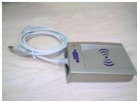
After you complete the installation for the software, Please connect the input line of the card issuer (encoder) with the USB port to your computer.
